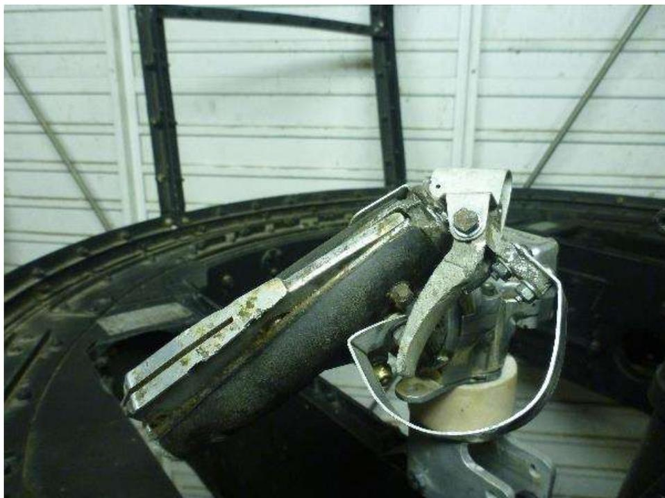
Then came that control shaft centre support and solenoid bracket. The one from my FN5 had been dismantled and (oddly) mostly flattened out. In some respects this turned out very convenient as it was now possible to do some CAD (Carboard Aided Duplication). Patterns were made for the parts before the FN5 bracket was re-built and then used to check for correct size and fit. Just need to make another one then.
