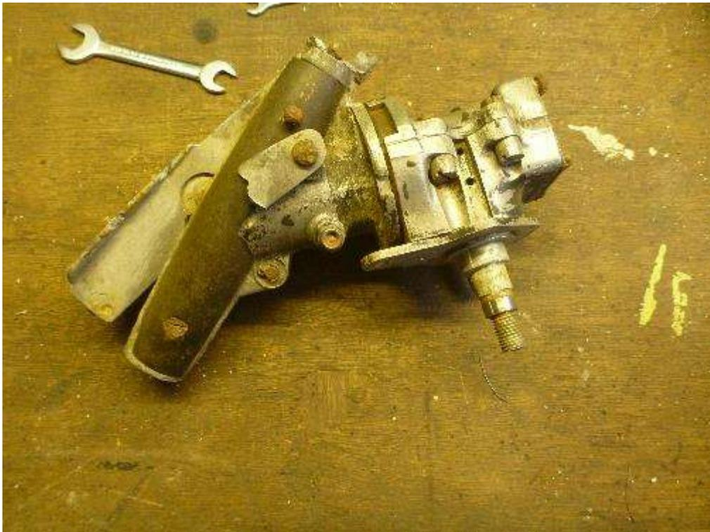
There was still the matter of the missing mounting bracket for the control handle. This was fabricated from alloy angle and took considerably longer than expected – in the order of three days! (The sharp eyed will notice it is fitted backwards, below)
