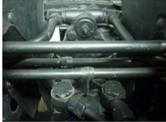
With the left side control handle, control rods and the control shafts all (hopefully) finally fitted, I turned my attention to the right side control handle. This apparently crash recovered handle was in a very poor state with many parts missing.
